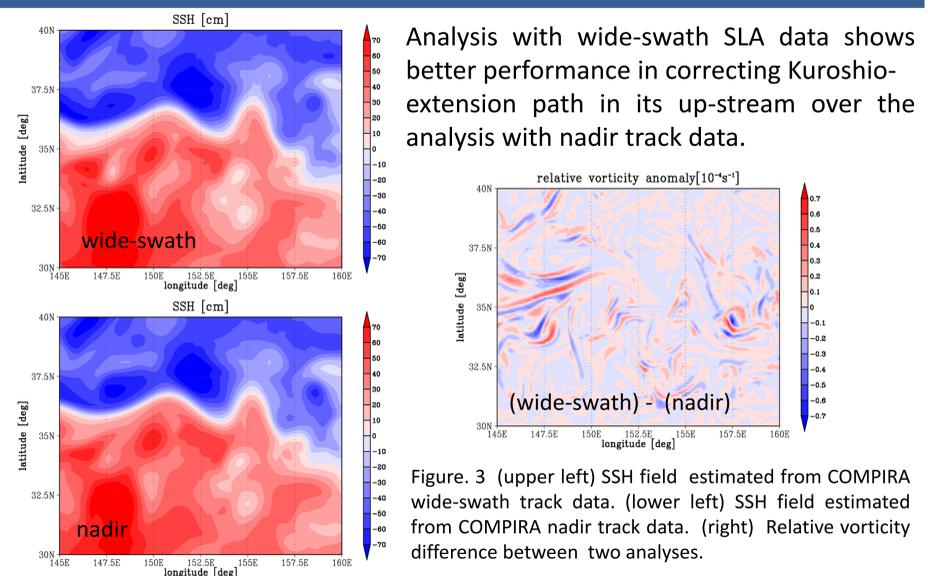
Figure. 3 (upper left) SSH field estimated from COMPIRA wide-swath track data. (lower left) SSH field estimated from COMPIRA nadir track data. (right) Relative vorticity difference between two analyses.
