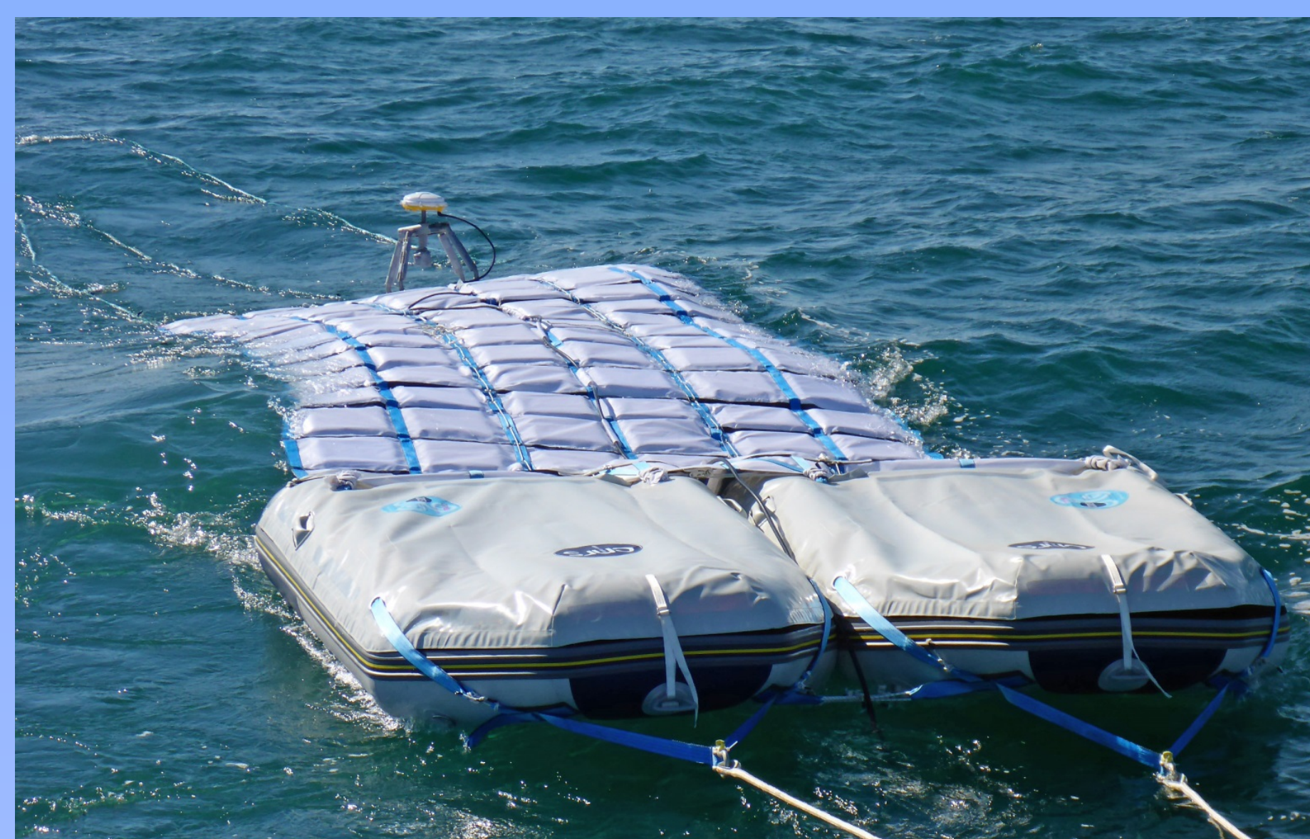
Drawing and towed GPS buoy at sea
