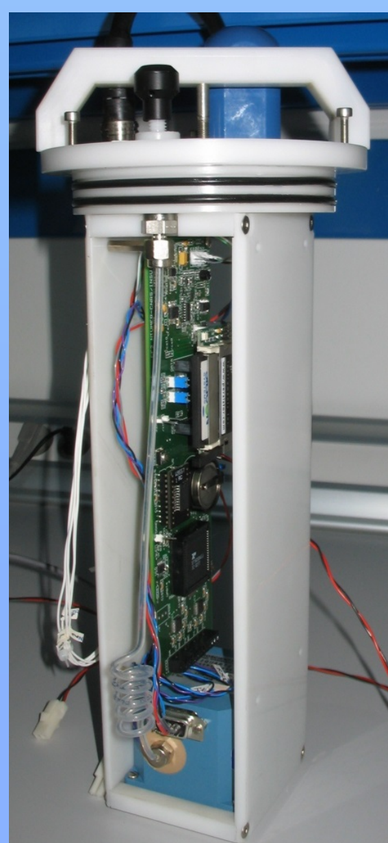
Inside of the tide recorder and multiparameter version
