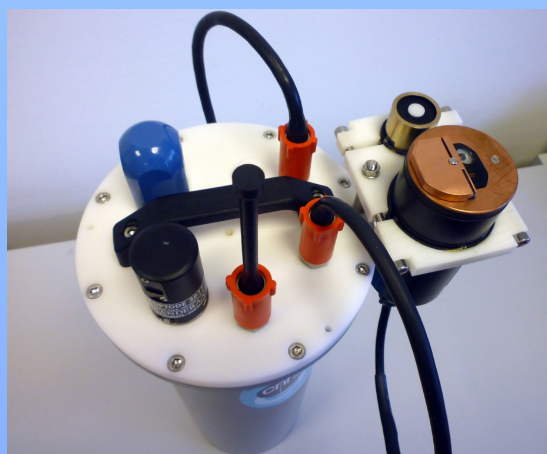
Inside of the tide recorder and multiparameter version
