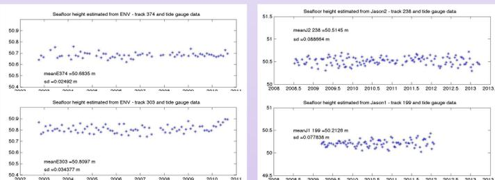
Seafloor height estimated at Sabine Bank tide gauge using Envisat data and Sabine tide gauge data. Hfloor374=50.68 +/- 0.02m. Hfloor303=50.81 +/- 0.03m
