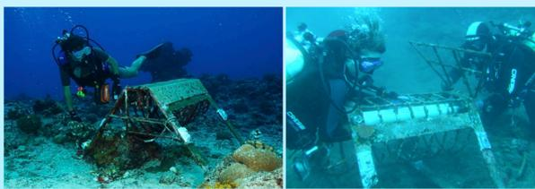
SBE26 and SBE26plus tide recorders are deployed for 1 to 2 year periods and calibrated at the manufacture between deployments when possible. They are installed in a fixed frame and replaced exactly in the same position each time.
