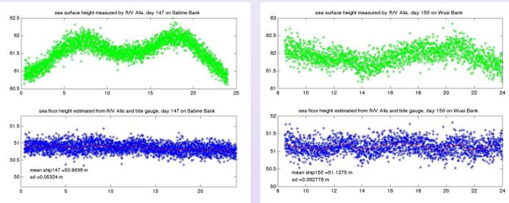
Sea surface and seafloor heights measured at Sabine Bank, using R/V Alis GNSS and Sabine tide gauge (day 147, 2010). Hfloor=50.86 +/- 0.05m
