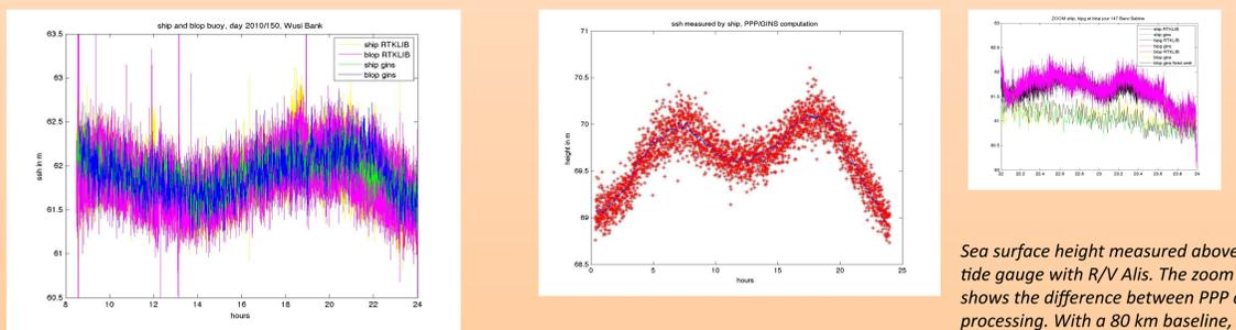
Sea surface height measured above Wusi tide gauge with R/V Alis and Blop buoy. In this case, double differences (DD) are noisier than PPP results, but are still reasonable.
