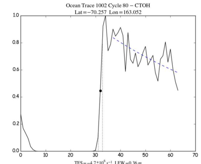
At CTOH, we processed the ERS-2 waveforms (WAP data) with a new implementation of the ICE-2 retracker algorithm, adding improvements and corrections to make it compatible and homogenous with the ENVISAT mission, hence providing suitable grounds for continuity and long-term altimetry data analysis. ESA recently released the REAPER product which represents the first version of GDR-like ERS product available globally (Femenias et al., 2014).
