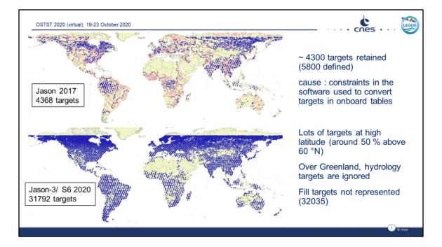
The 2017 generation for Jason-3 was conservative as the altimeter on Jason-3 can switch very rapidly between Close Loop (CL) and Open Loop (OL) modes (in less than 1 second). Then, it is not necessary to define hydrology target everywhere over land. When no hydrology target is defined the altimeter switches automatically in CL mode. The hydrology targets were then generated for Jason-3 only where we already had a good knowledge of the position and the elevation of the waterbodies.
