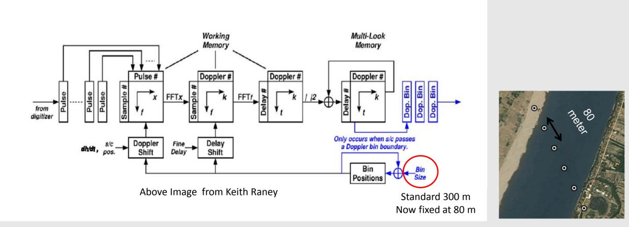
In the Delay-Doppler Scheme, the only change that we operate regards the grid bin size: **WE DONT CHANGE THE THEORETHICAL ALONG TRACK RESOLUTION, ONLY THE GRID STEP SIZE!**
