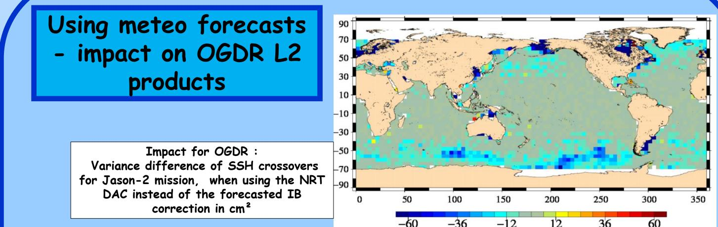
The availability of ECMWF meteorological forecasts daily allows producing DAC forecasts daily on the same time span; it is named DAC NRT/OGDR. Using the forecasted DAC instead of the IB allows reducing significantly the altimeter variance (cf. figure above for 1 year of Jason-2 L2 data). This NRT DAC is generated operationally since september 2013 and it is used in <u>DUACS products only</u> at present time.
