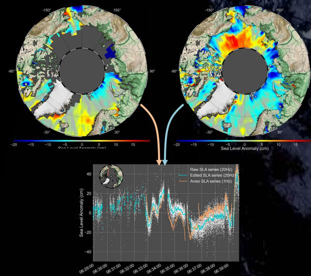
Fig. 1: Upper panel, gridded SLA SARAL/AltiKa over cycle 7, computed with Aviso (Left) and CLS/PML Arctic (Right) data. Lower panel, Along-track SARAL/AltiKa SLA (Cycle 7/Pass 2) with raw (white) and final (blue) 20Hz CLS/PML Arctic product and Aviso (orange) product.
