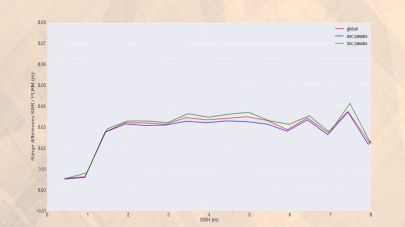
SAR / P-LRM range differences exhibits a constant 3 cm bias for most of the waves. Different behavior is observed for low SWH (below 1 m).
