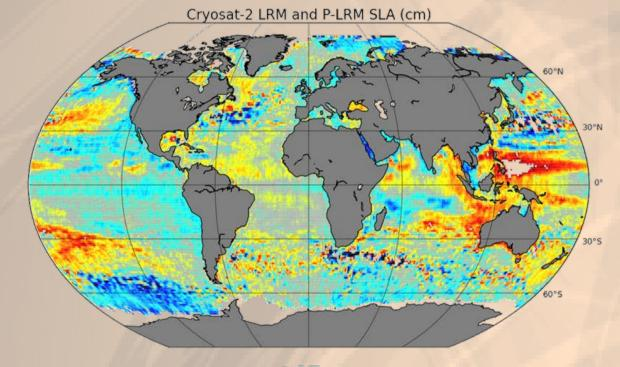
Analysis of continuity as function of the latitude around the equatorial Pacific SARM box shows differences lower than 1cm
