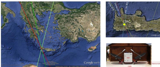
CDN1: A permanent altimeter calibration site with a transponder in West Crete, Greece.
