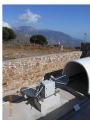
Transponder deployment at CDN1 site is complete. All instruments and devices are controlled remotely via satellite and 3G communication links.
