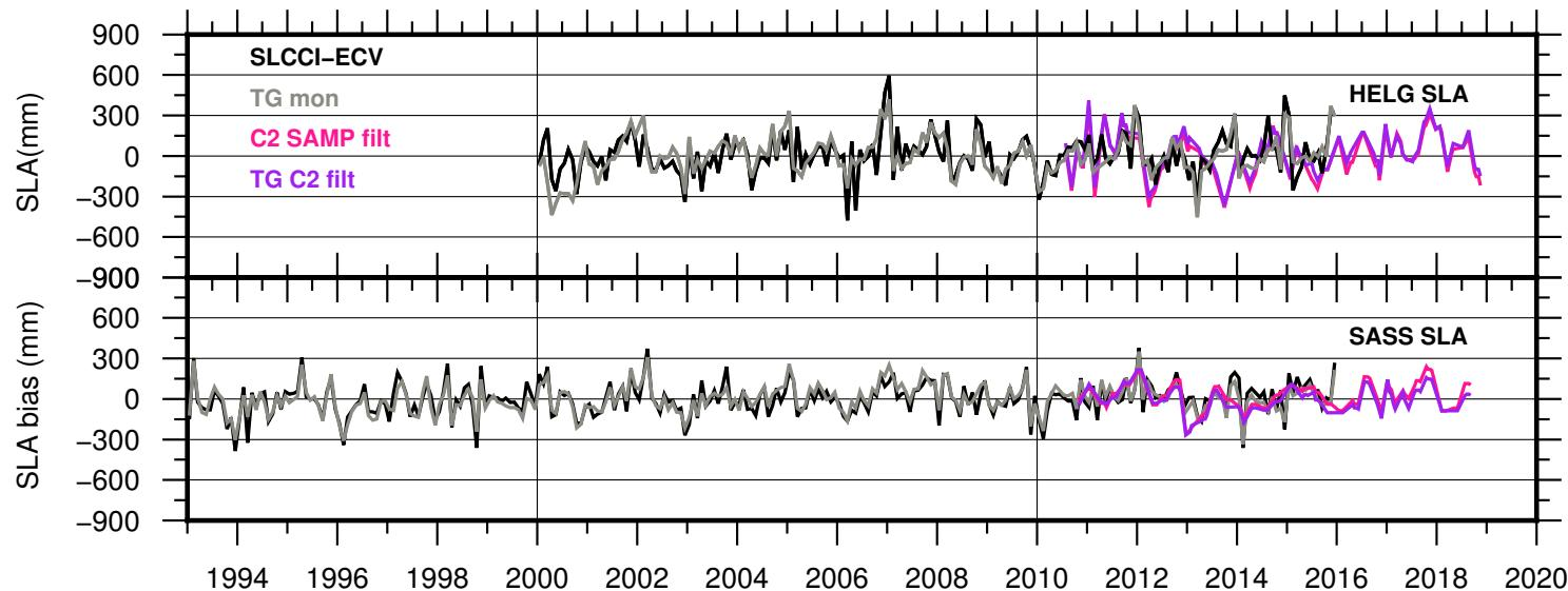
**Fig. 7.** Sea level time-series from in-situ data, multi-mission altimetry (SLCCI) and from CryoSat-2 at Helgoland (top) and Sassnitz (bottom) over the complete altimeter period 1993-2019. The filtered CryoSat-2 time-series correspond to the nearest point (C2 SAMP filt). In-situ data are the monthly records and the filtered time-series corresponding to C2 SAMP filt.
