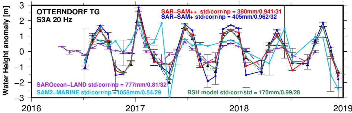
**Fig. 3.** Figures include comparison with ocean models. The std of model with TG is 17-18 cm at both locations.
