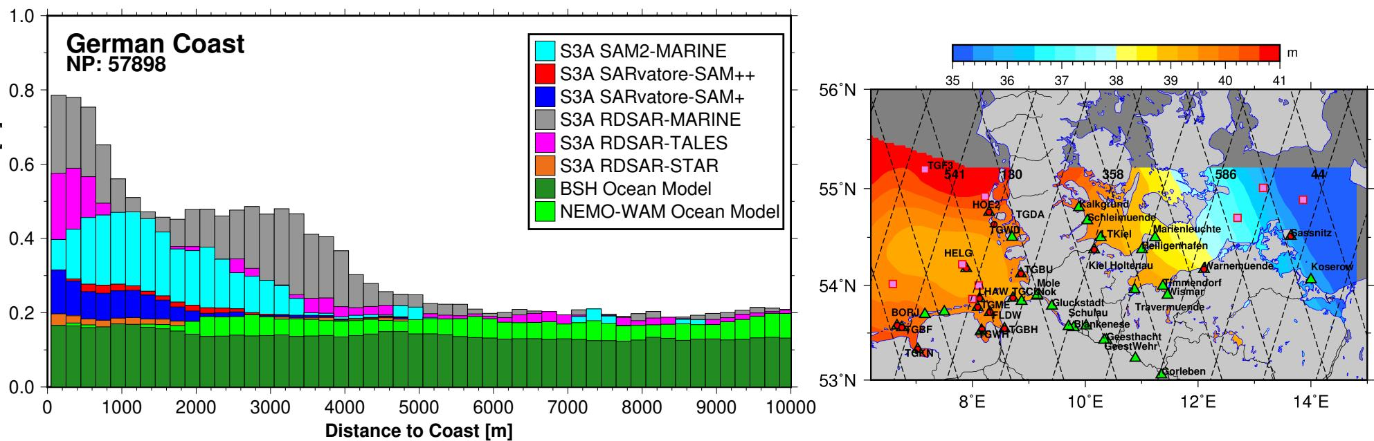
**Fig. 1.** Standard deviation of sea surface height anomaly in the GEC for altimeter products and ocean model. Sentinel-3.A from June 2016 to Dec. 2018. BSH and NEMO-WAM corrected for ocean tide model TPX08. NP is the number of meas..
