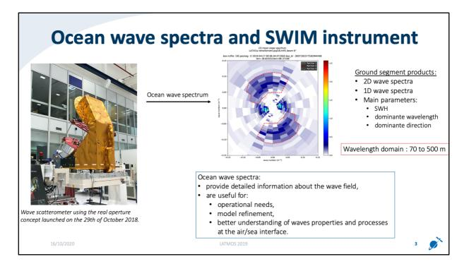
SWIM is the first space wave scatterometer that uses the real aperture concept. It allows to compute ocean wave spectra which give very detailed information about the wave filed. SWIM measures wave with wavelengths between 70 and 500 m.
