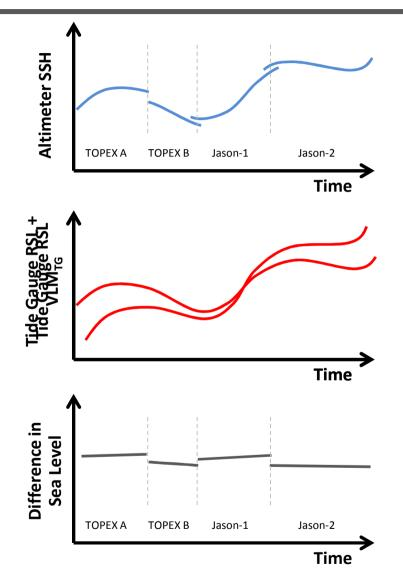
For any given comparison point, we form the difference in sea level (corrected for vertical land motion, VLM, using one of a few different strategies) and then parameterise:
