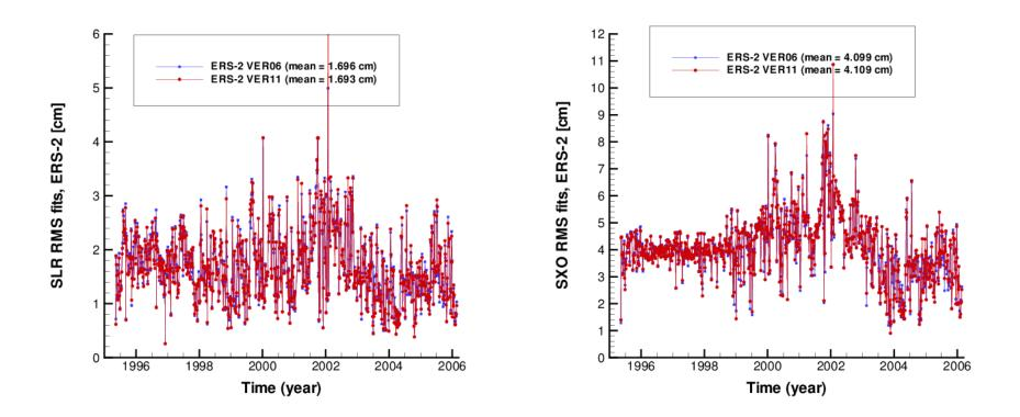
The mean value of the SLR RMS fits reduced from 1.696 to 1.693 cm,
