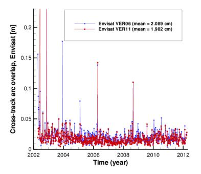
Reduction of the mean values of the arc overlap of VER11 orbit, as compared to VER06 orbit: Radial – from 0.517 to 0.534 cm, i.e. by -0.017 cm (about -3.2%), Cross-track – from 2.089 to 1.982 cm, i.e. by 0.107 cm (about 5.1%), Along-track – from 2.140 to 1.933 cm, i.e. by 0.207 cm (about 9.7%)
