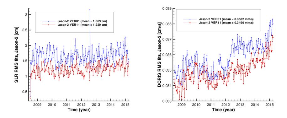
The mean value of the SLR RMS fits reduced from 1.663 to 1.229 cm,
