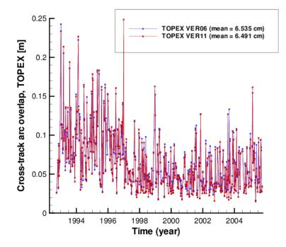
Reduction of the mean values of the arc overlap of VER11 orbit, as compared to VER06 orbit: Radial – from 1.023 to 0.890 cm, i.e. by 0.133 cm (about 13.0%), Cross-track – from 6.535 to 6.491 cm, i.e. by 0.044 cm (about 0.7%), Along-track – from 3.593 to 3.476 cm, i.e. by 0.117 cm (about 3.3%)
