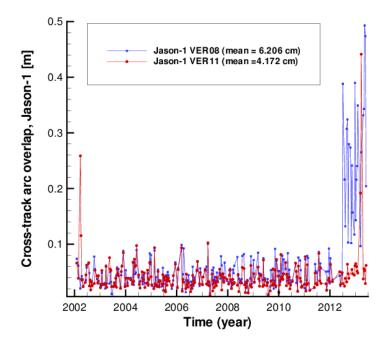
Reduction of the mean values of the arc overlap of VER11 orbit, as compared to VER08 orbit: Radial – from 0.979 to 0.785 cm, i.e. by 0.194 cm (about 19.8%), Cross-track – from 6.206 to 4.172 cm, i.e. by 2.034 cm (about 32.8%), Along-track – from 4.580 to 2.482 cm, i.e. by 2.098 cm (about 45.8%)!
