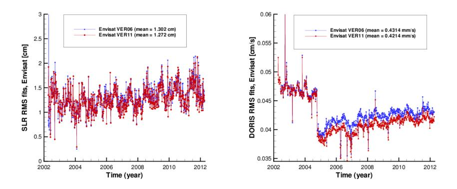
The mean value of the SLR RMS fits reduced from 1.302 to 1.272 cm,
