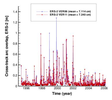
Change of the mean values of the arc overlap of VER11 orbit, as compared to VER06 orbit: Radial – from 1.836 to 1.852 cm, i.e. by +0.016 cm (about +0.9%), Cross-track – from 7.114 to 7.240 cm, i.e. by +0.126 cm (about 1.8%), Along-track – from 10.690 to 10.632 cm, i.e. by -0.058 cm (about -0.5%)
