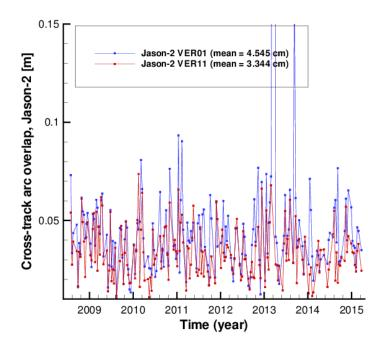
Reduction of the mean values of the arc overlap of VER11 orbit, as compared to VER01 orbit: Radial – from 0.782 to 0.558 cm, i.e. by 0.224 cm (about 28.6%), Cross-track – from 4.545 to 3.344 cm, i.e. by 1.201 cm (about 26.4%), Along-track – from 3.657 to 1.456 cm, i.e. by 2.201 cm (about 60.2%)
