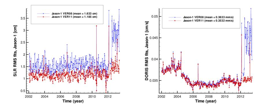
The mean value of the SLR RMS fits reduced from 1.633 to 1.185 cm,
