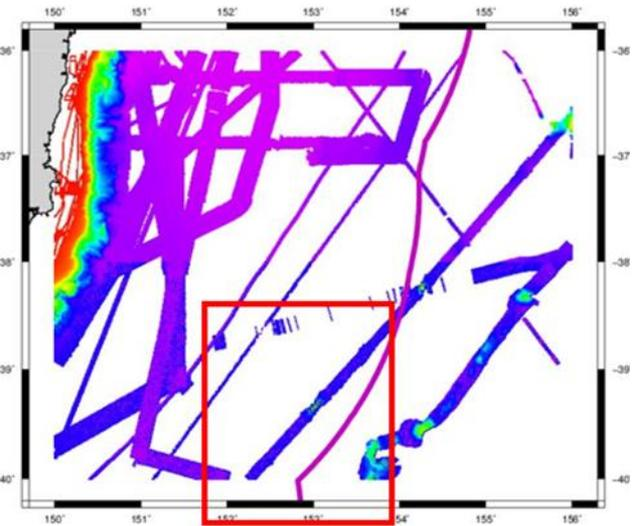
Tiles of the DEM50m from Geoscience Australia are composed of discontinuous bathymetric surveys. In some cases, artefacts appear when integrating some of the DEM50m tiles in the initial bathymetry. Although the DEM50 dataset is more recent than the initial bathymetry, some tiles were discarded from the integration.
