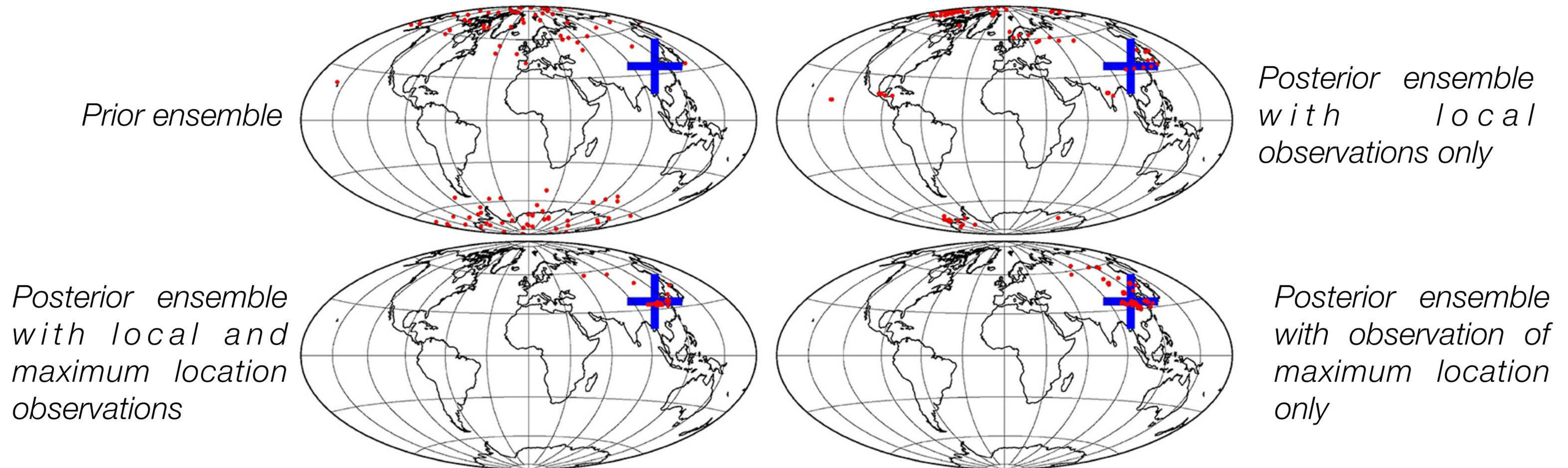
*Figure: Blue cross: location of maximum in the true field. Red dots: ensemble members. This experiment illustrates the capability of the algorithm to deal with the non-local observation of the maximum location.*
