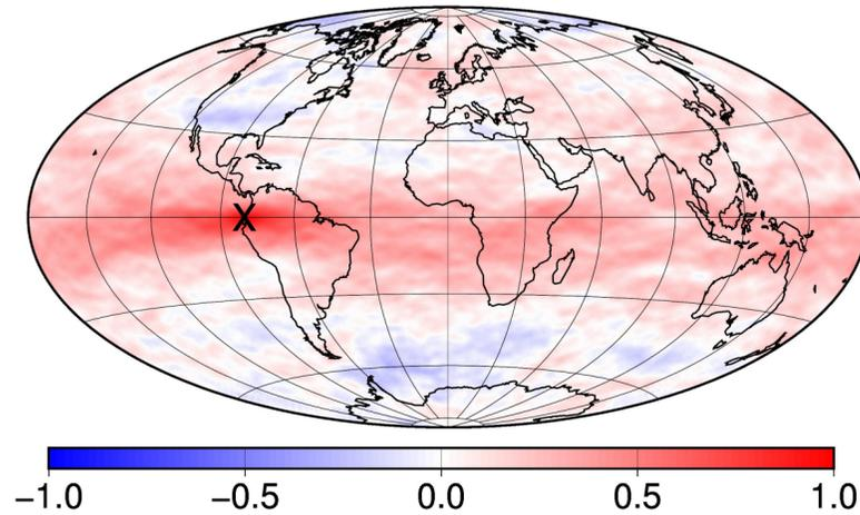
*Fig 4: Correlations  $C$  localized by Schur-multiplying with  $C_4$*
