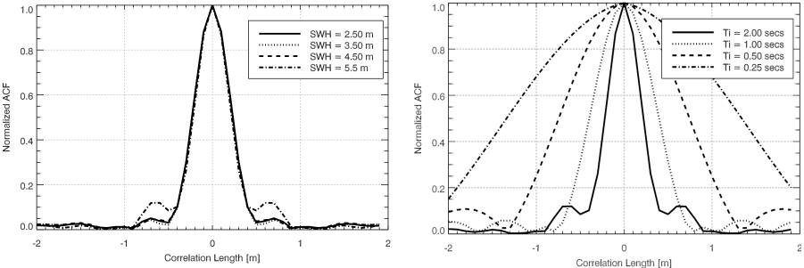
Thus FF-SAR can get statistically independent looks at the ocean every ~0.5 m along track, or ~13,500 per second. [Almost. The lacunar sampling of closed burst mode causes some small degradation in this, by introducing small side lobes in the along-track PTR.]
