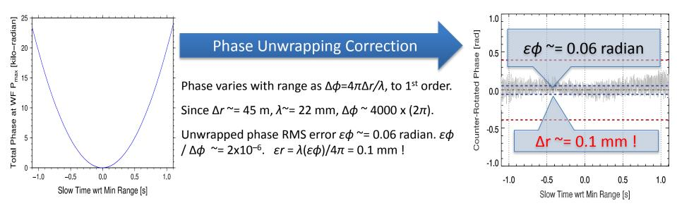
If the FF-SAR calculation employs the maximum possible aperture length ( $T_1 = T_{vis}$ ) then it must undo phase changes of the order of 4000 cycles of  $2\pi$ . After doing this, the residual phase error in each pulse echo is about 0.06 radian, only 2 parts per million of the total change in phase occurring across the aperture. (FF-SAR requires a theory of phase more accurate than just the first-order effect. We account for higher-order effects.)
