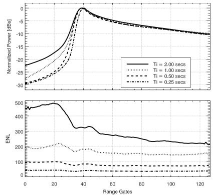
The mean waveform shape depends on the coherent integration time  $T_i$ .  $T_i$ i = 2 s gives a broad "toe" about 23 dB below peak. Reducing  $T_i$  makes the rise steeper and brings the toe down 30 dB below peak.
