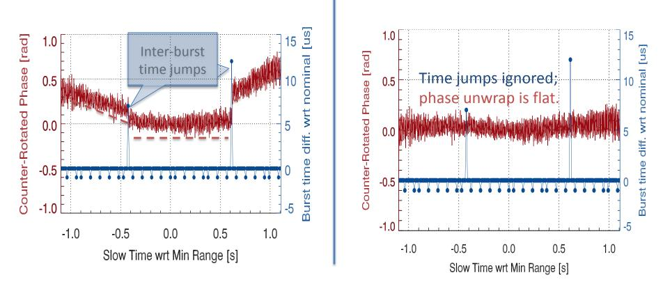
Datation errors of a few microseconds are enough to spoil focus. FF-SAR over a transponder proves that the radar is running steadily even when the datation in the data product shows a jump of a few micro-seconds. To achieve optimal focus we had to correct the datation.
