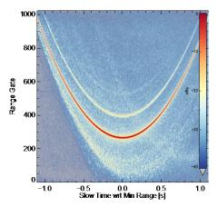
As a radar flies over a fixed point on the Earth, the range (oneway distance) to that point changes from echo to echo. Looking through the instrument's range window at a sequence of pulse echoes, the ground point traces a parabolic trajectory. The total time that the point is "visible" to the radar,  $T_{vis}$ , depends on how long the point stays in the window. For CS2 & S3,  $T_{vis}$  is ~2 seconds for points near the ground track.
