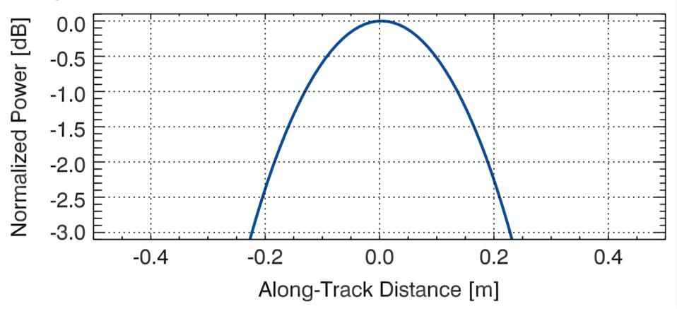
Cryosat SAR FBR data over the Svalbard transponder on 6 May 2014.  $T_I = T_{vis}$ . Moving the focal point along-track by a fraction of a meter changes the coherently integrated power. This along-track point target response has full width at half maximum of only 0.45 meter.
