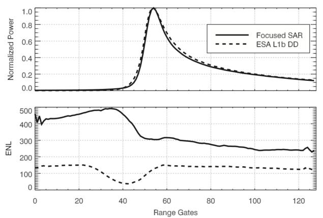
20 Hz, so the two can be compared, the mean waveforms of FF-SAR and unfocused D/D SAR (Cryosat L1b) have similar shapes. FF is a little more peaked. The main advantage is that FF ENL is higher than D/D ENL by a factor of 2 to 3, depending on range gate.
