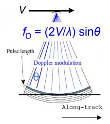
Increasing  $T_i$  decreases  $\Delta f_D$ , narrowing the Doppler beam and narrowing the resolution of  $\theta$ , improving the sensitivity to along-track position.
