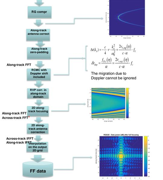
**WK** Omega-k (WK) algorithm is based on the idea that the exact transfer function can be written in a closed-form expression using the Stationary Phase principle
