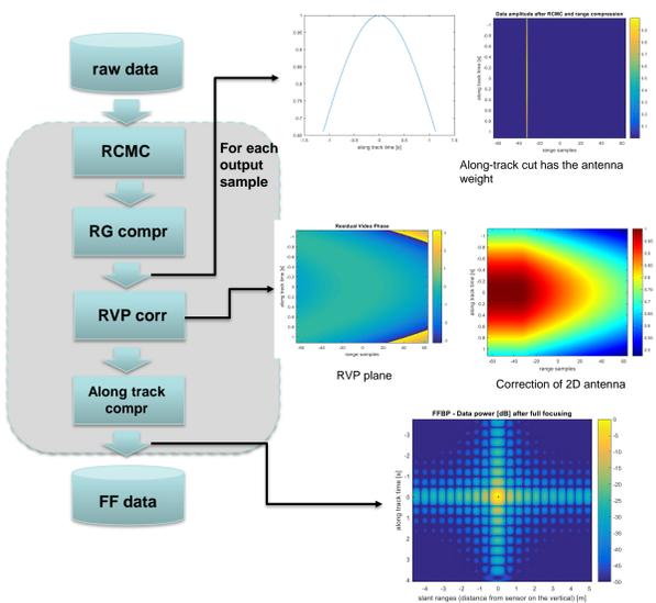
**RGD2D** It is based on Range-Doppler algorithm: azimuth focusing is performed in the transformed domain
