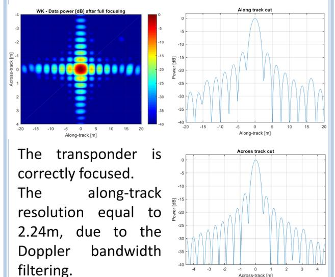
The transponder is correctly focused. The along-track resolution equal to 2.24m, due to the Doppler bandwidth filtering.
