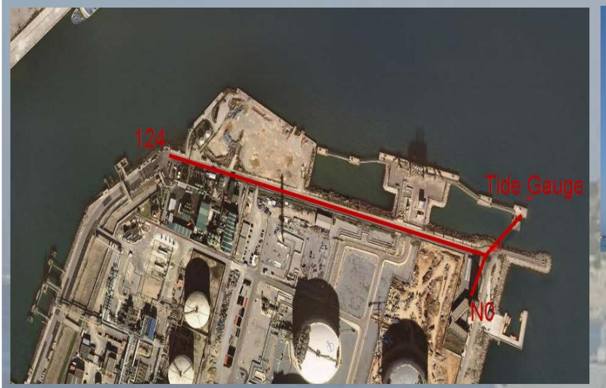
. General view of the levelling traverse conducted in 2009 and repeated in September 2011 (red line, *about 700 m along the northern* side of the "Energy Pier", Barcelona harbour, Spain). The levelling chain links point #124 (Levelling Network XdA), the Tide Gauge (point #146) and the Harbour Control Tower (NO point is located at the ground floor of the Tower, whereas the GPS Station- ARP point- is at its roof). Source of the orthophotomap: Institut Cartogràfic I Geologic de Catalunya (ICGC).
