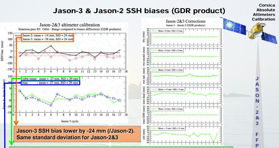
Most of the SSH bias differences come from the orbit-range (-23 mm) suggested that most of the Jason-3 and Jason-2 SSH biases difference comes from the range.
