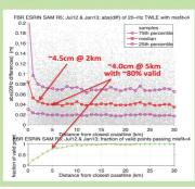
The figure (left) shows 20Hz noise on Total Water Level Envelope (TWLE) for Cryosat-2 SAR data around the UK, as a function of distance to the closest coast (shown in figure below). TWLE is the sea level inclusive of tides and pressure/wind effects.
