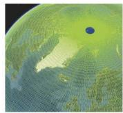
CryoSat-2 ground tracks for one sub-cycle (29 days)
