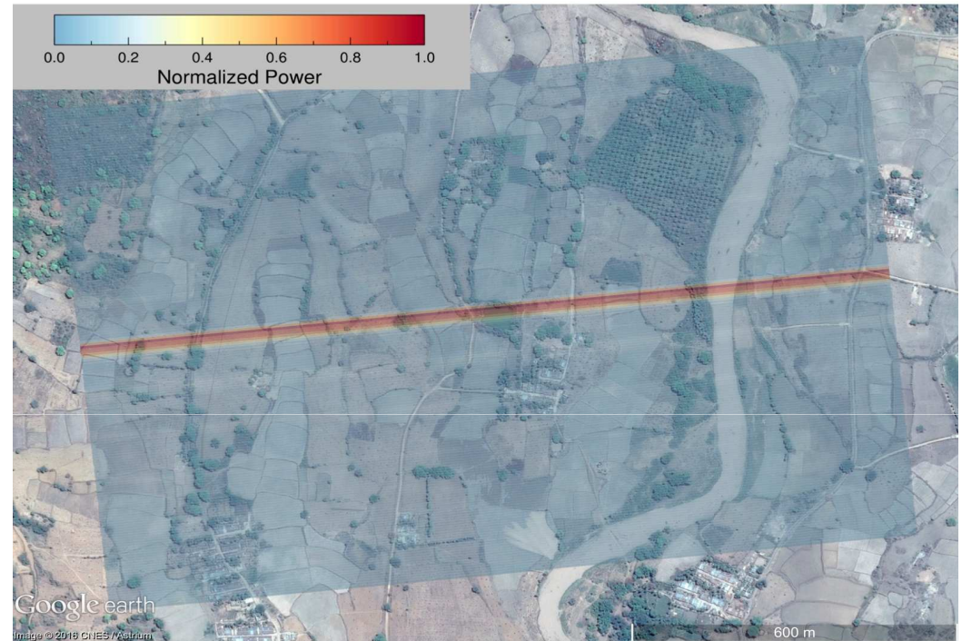
Fully-Focused SAR Response over the pond. Normalized Power in color scale. Rectangles represent the FF SAR altimeter footprint, \sim 5 m along-track by \sim 1500 m across-track
