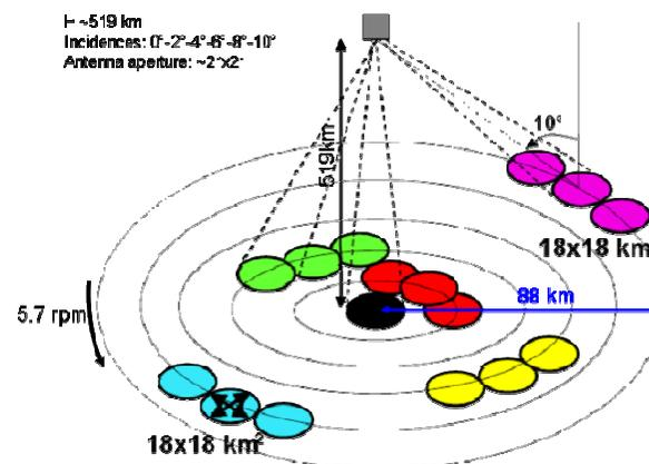
Alternate six beams illumination with  $360^\circ$  rotation
