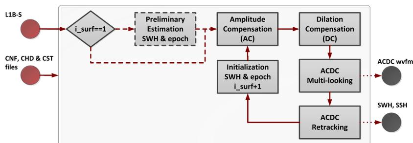
**Initial estimates (first surface)** of **SWH & epoch** performed with **in-house implementation of the fully analytical SAR ocean model** (Chris Ray et al 2015, see [2]) → **synergy with L1B processing**
