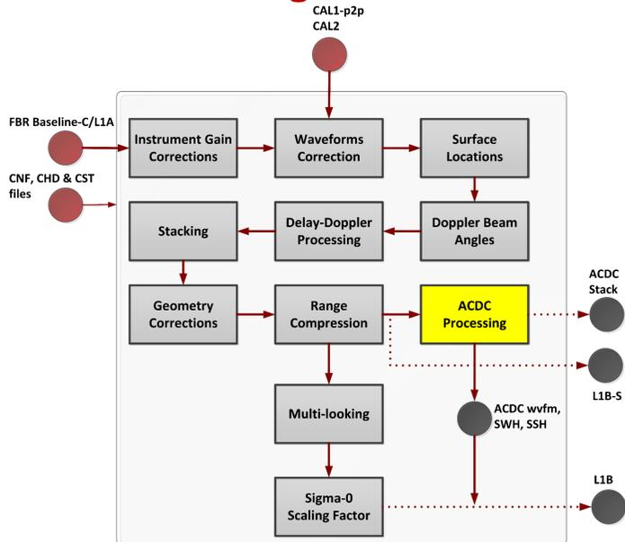
DDP structure change with stacking before geometry corrections allows an **easy integration of ACDC processing** → **conventional + ACDC stack (L1B-S)** are provided as optional products.
