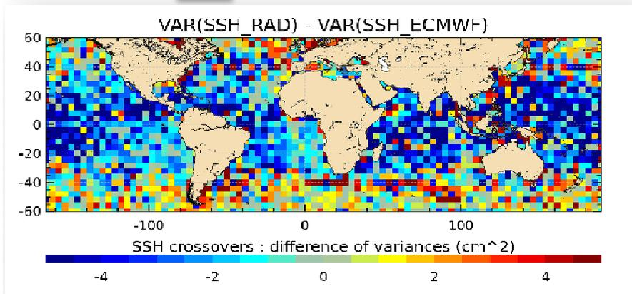
Quality of wet tropospheric correction (WTC) is evaluated by differences of variances of SSH at Xovers (radiometer vs ECMWF WTC)
