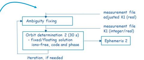
The final measurement file can be used in other configurations
