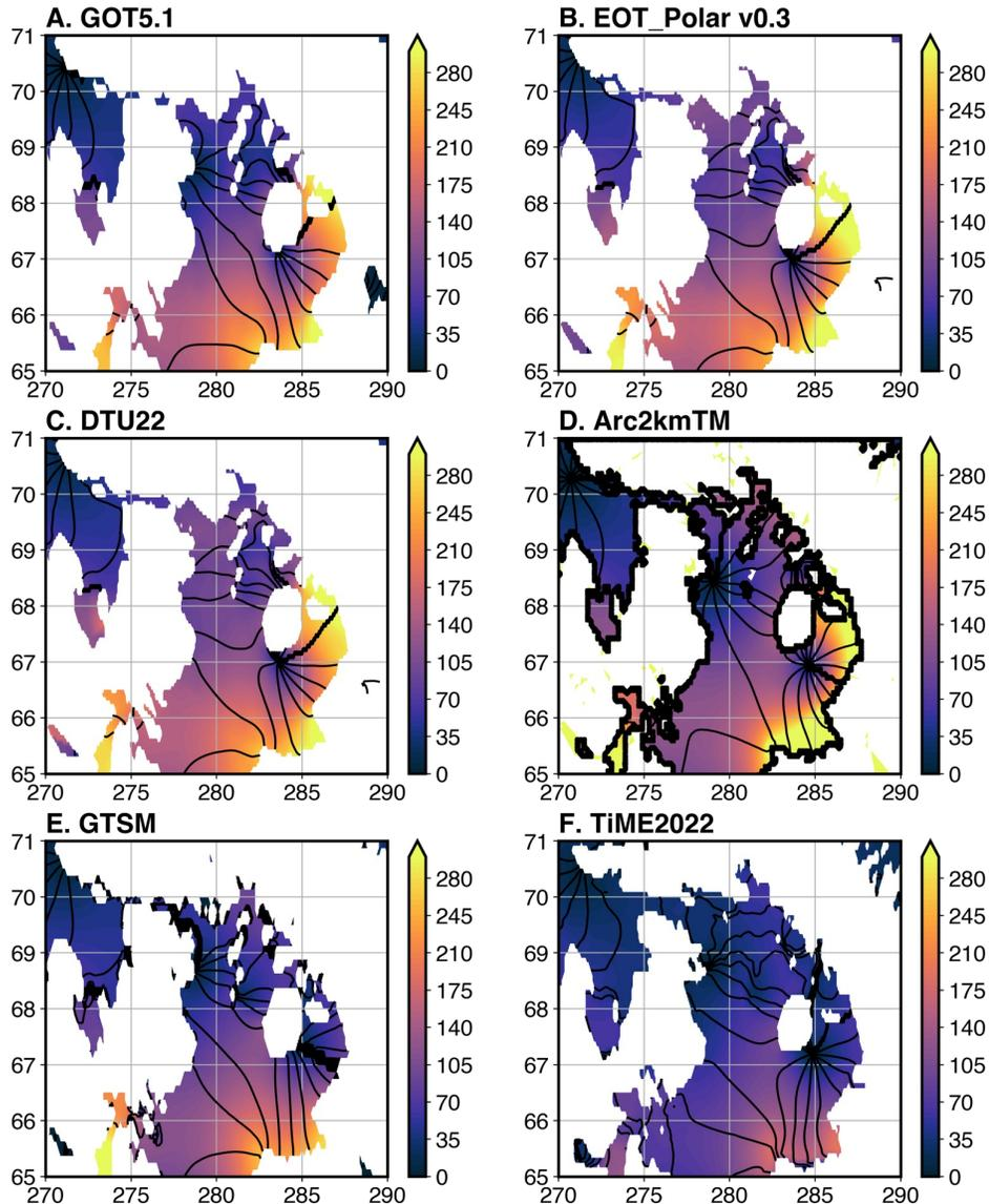
**Figure.**  $M_2$  for 6 models, three semi-empirical and three numerical models. EOT (Hart-Davis et al 2021 updated), GOT (Ray 1999 updated) and DTU (Andersen et al 2023) all include Cryosat-2.
