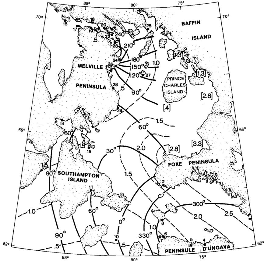
Figure 12.7.  $M_2$  co-tidal chart for GMT + 4 hr time zone. Co-phase (deg.) represented by solid lines and co-amplitude (m) by dashed lines. Smaller numbers indicate station numbers whose data (Table 12.1) is used to plot chart. Large numbers in square brackets are reported tidal amplitudes (no phases).
