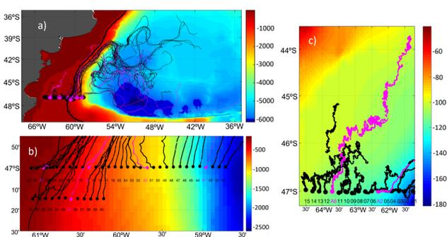
Figure 1: Trajectory of the 62 drifters deployed. Large dots correspond to the initial position. 55 custom drifters correspond to black lines; 7 magenta lines correspond to drifters provided by NOAA. In the background the topography is represented (m, IOC,2003). The 200m isobath is indicated with a black width line. (a) shows the complete trajectories; (b) shows a zoom for the drifters located over the continental slope and (c) shows a zoom over the continental shelf.
