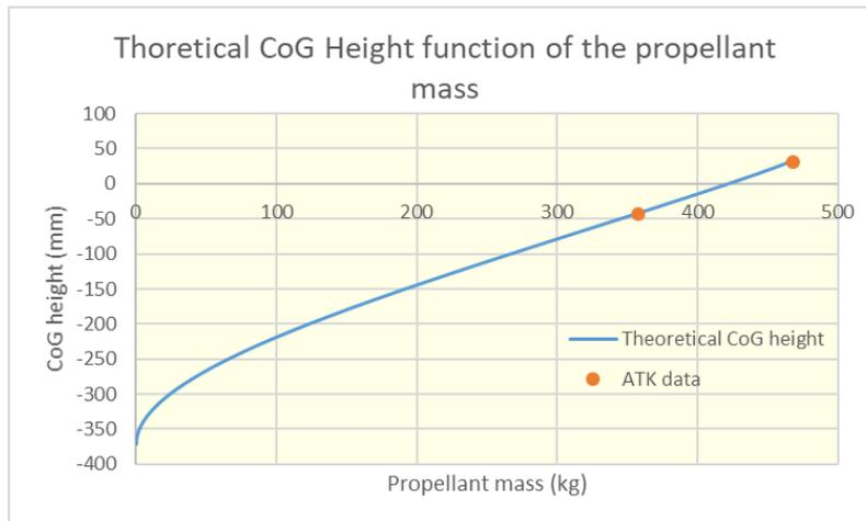
Figure 10 : Resulting analytical evolution of the propellant center of mass function of remaining mass in the tank. Comparison with tank supplier committed data confirms representativeness.
