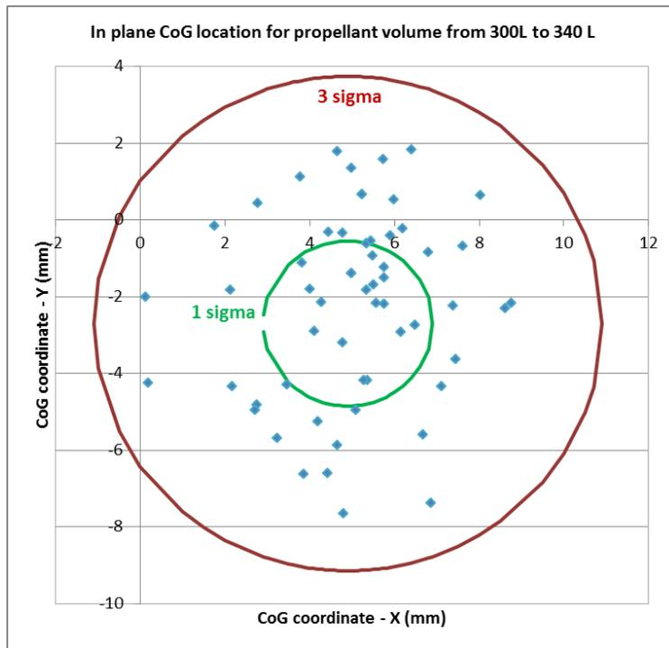
Figure 13: In-plane propellant center of mass location distribution for 20 repetitions, for filling ratio consistent with SWOT science mission ranges. 1sigma and 3 sigma unbalances can be defined.
