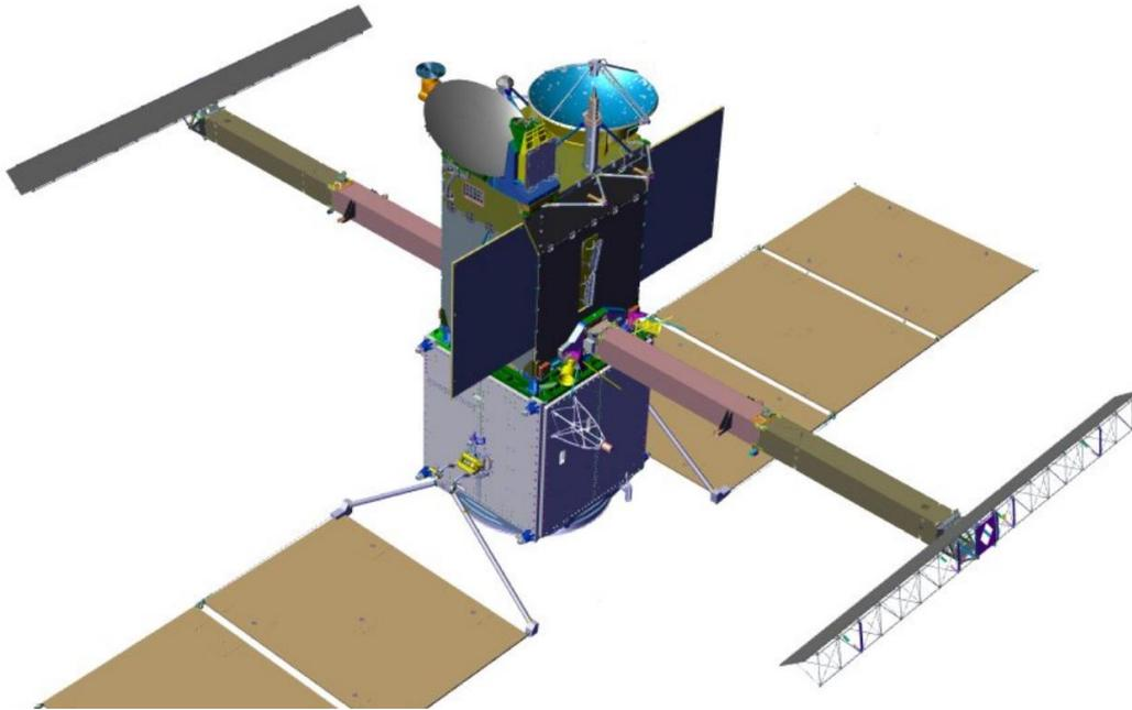
Figure 2. Payload module on the top of SWOT satellite
