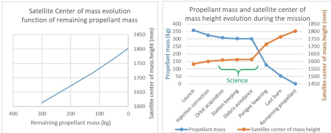
Figure 6 : Left : satellite center of mass function of remaining propellant mass. Right : Propellant mass and satellite center of mass height evolution along the mission illustrates the need for modelling to retrieve accurate POD during the science mission
