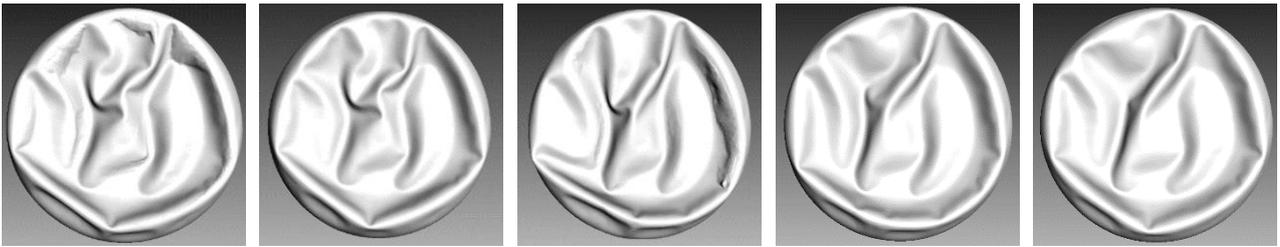
Figure 12: Diaphragm surface scans for same filling ratio (340L) for 5 different repetitions from ATK SWOT dedicated tests.
