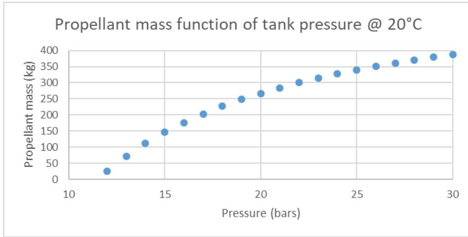
Figure 7 : Propellant mass function of flight nitrogen pressure measurement @ 20°C
