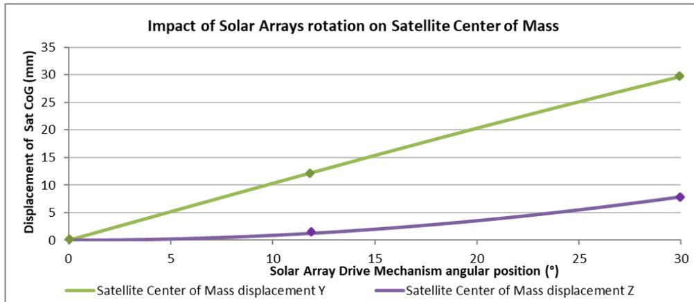
Figure 16 : when solar arrays orientation is shifted to follow season, the satellite center of mass is impacted significantly.
