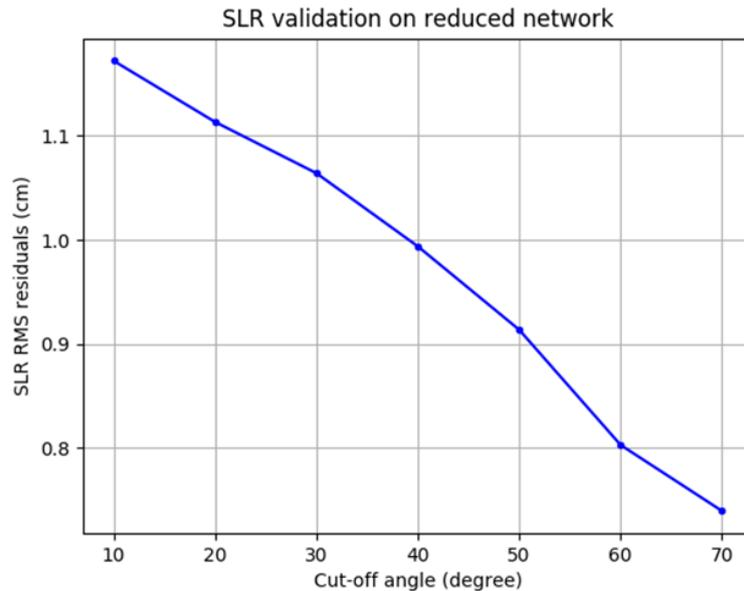
Figure 23– Estimation of Satellite Laser Ranging residuals versus elevation (against Doris+GPSP CNES orbit solution)
