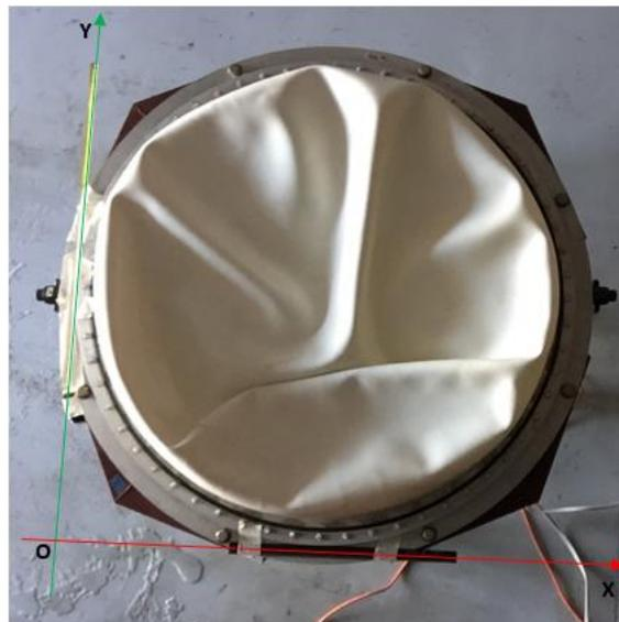
Figure 11 : SWOT tank diaphragm. It illustrates stiffness and non-flat surface at partial filling ratio.
