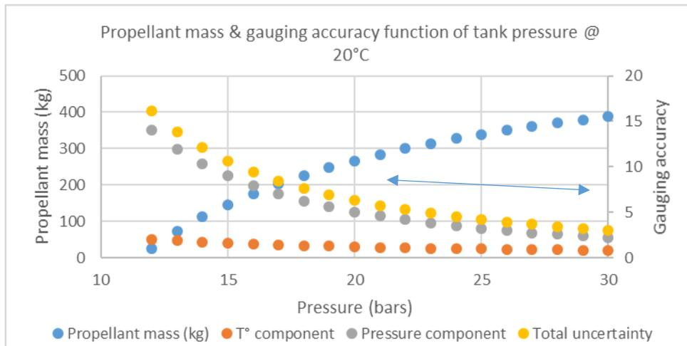
Figure 8 : Propellant mass and gauging accuracies identifying components due to T° measurement uncertainty and pressure measurement uncertainty. Performance is only required for science mission.
