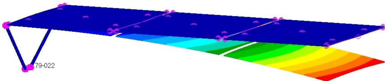
Figure 21 : Representation of the SWOT’s solar array deformed when it’s loaded by a thermal gradient across wing. To make the view comprehensible, the deformed wing doesn’t respect the real scale.
