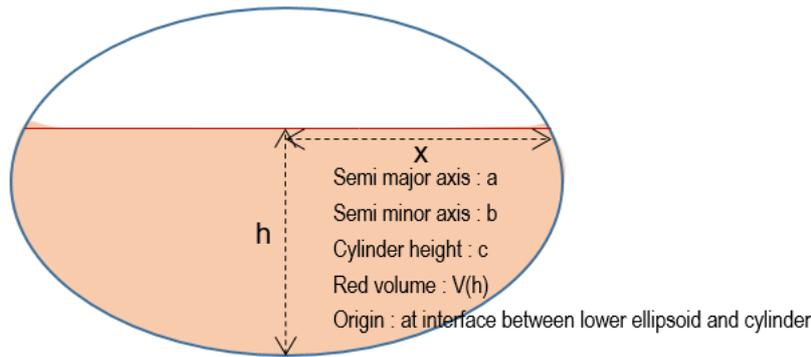
Figure 9 : Schematical representation of the propellant shell, with geometry justifying the analytical mass, volume and center of mass derivation.
