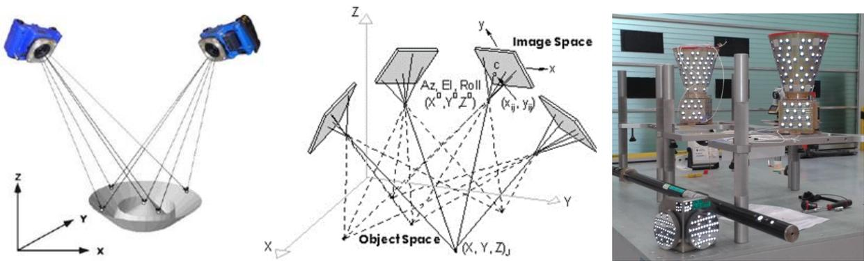
Figure 20 : Photogrammetry uses multiple photographs from different view point (left). Triangulation from all photographs is performed to retrieve object location (middle). Objects are equipped with dedicated targets (right)
