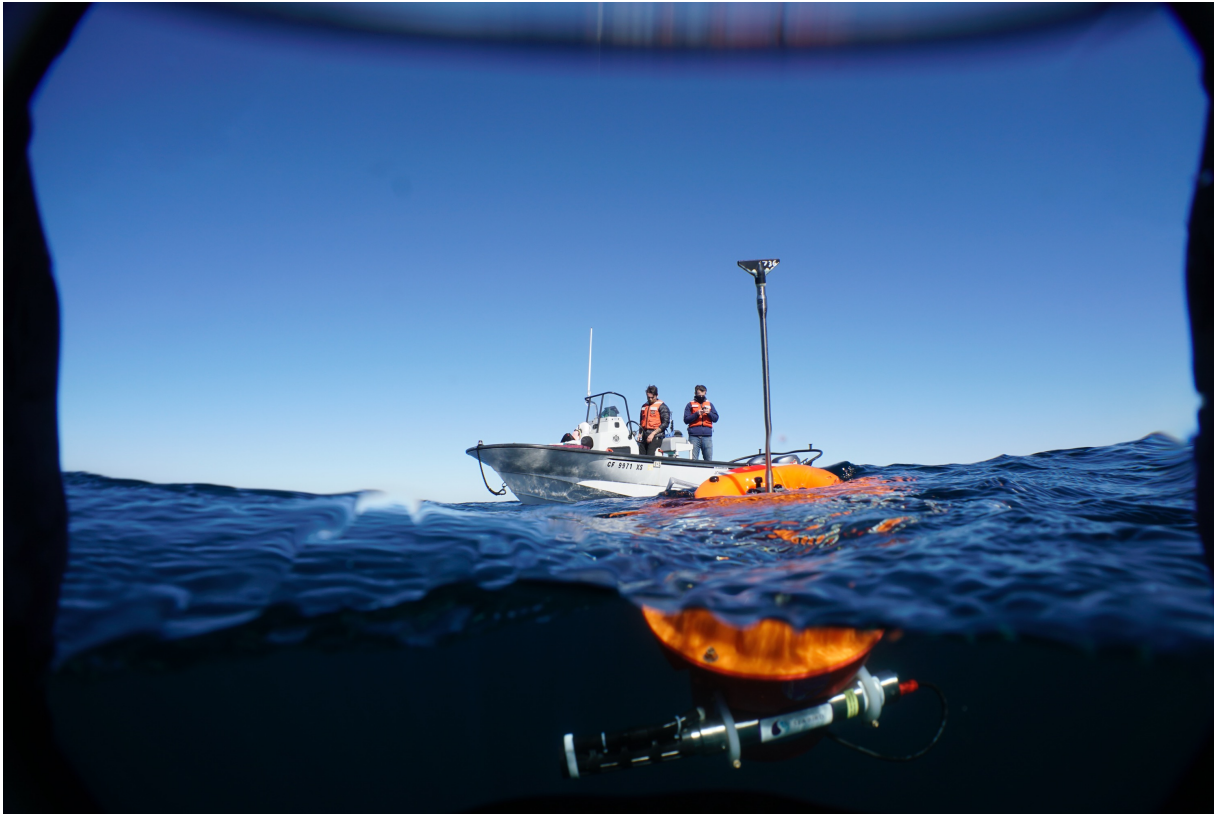
Testing of the SBS61 on the Deep SOLO float by the Scripps Argo lab
