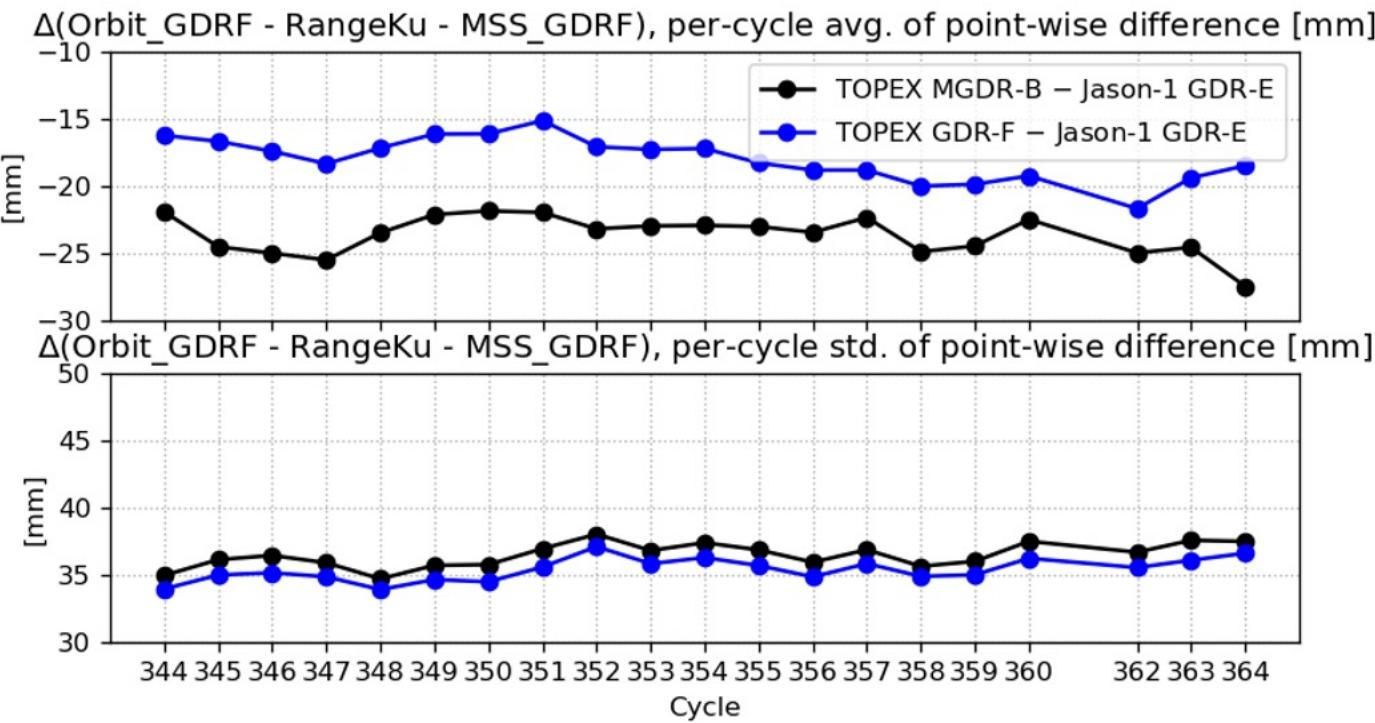
Numerical Retracking improves consistency with Jason-1
