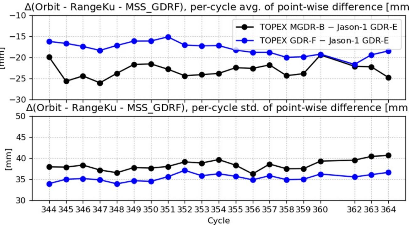
**Improved orbit solution is improving the consistency (stability of averages and reduction of stddev) of the difference.**
