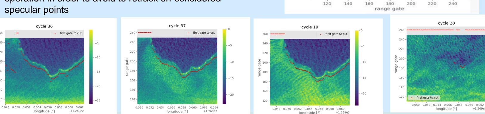
mean power of each population. We can observe a 3dB loss between sea and ground (division by 2 in watts). This fact indicate that the ground does not backscatter signal (because we still get the oceanic signal from the other side of the track). The specular mean value is often very high and close to the max (0dB)
