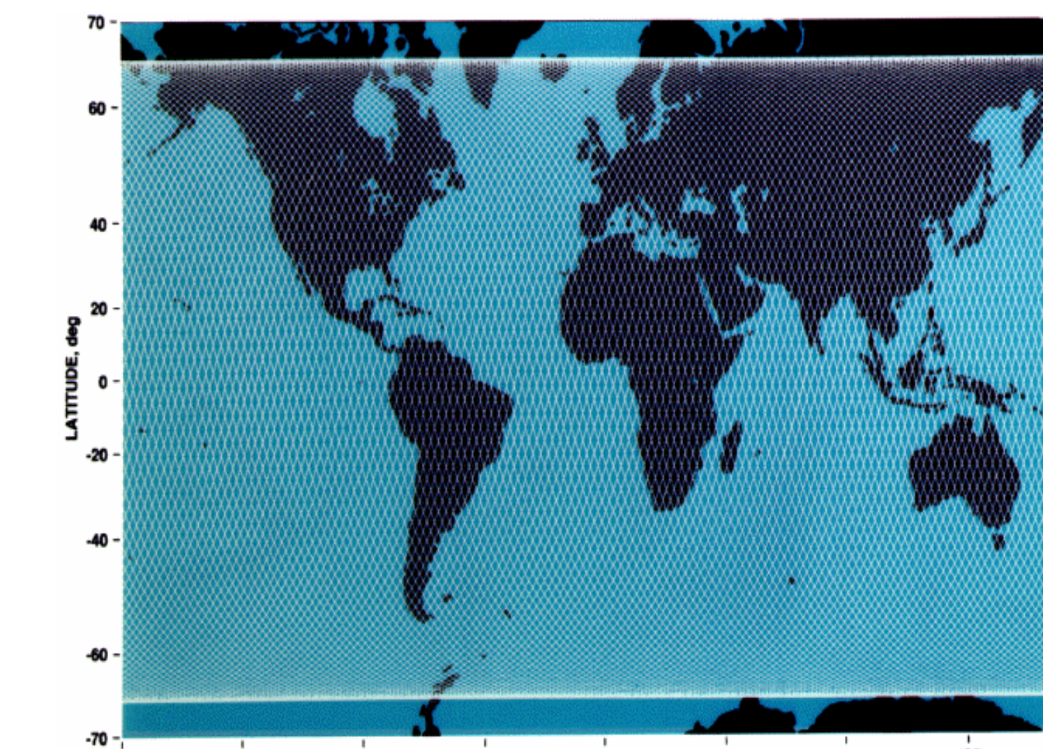
Jason-3 ground track coverage every 10 days which is the same orbital path as Jason-2 before 2-Oct-2016
