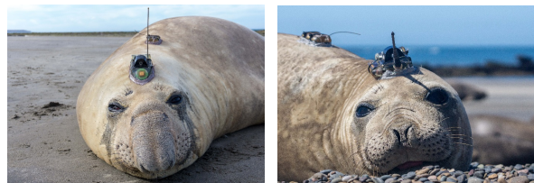
Figure 2: Left: Female equipped in October 2021 with a CTD-Oxygen oceanographic tag designed by the Sea Mammal Research Unit as part of the H2020 Nautilus project. Right: Elephant seal male equipped in October 2021 by a CTD-GPS Oceanographic tag.
