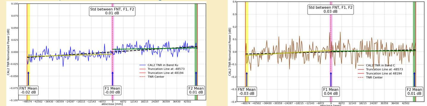
CAL2 Thermal Noise Response (TNR) in blue for Ku-Band (left) and in brown (right) for C-Band in case of side-A. The slope of the TNR is only 0.02 dB end-to-end and std around 0.01 dB
