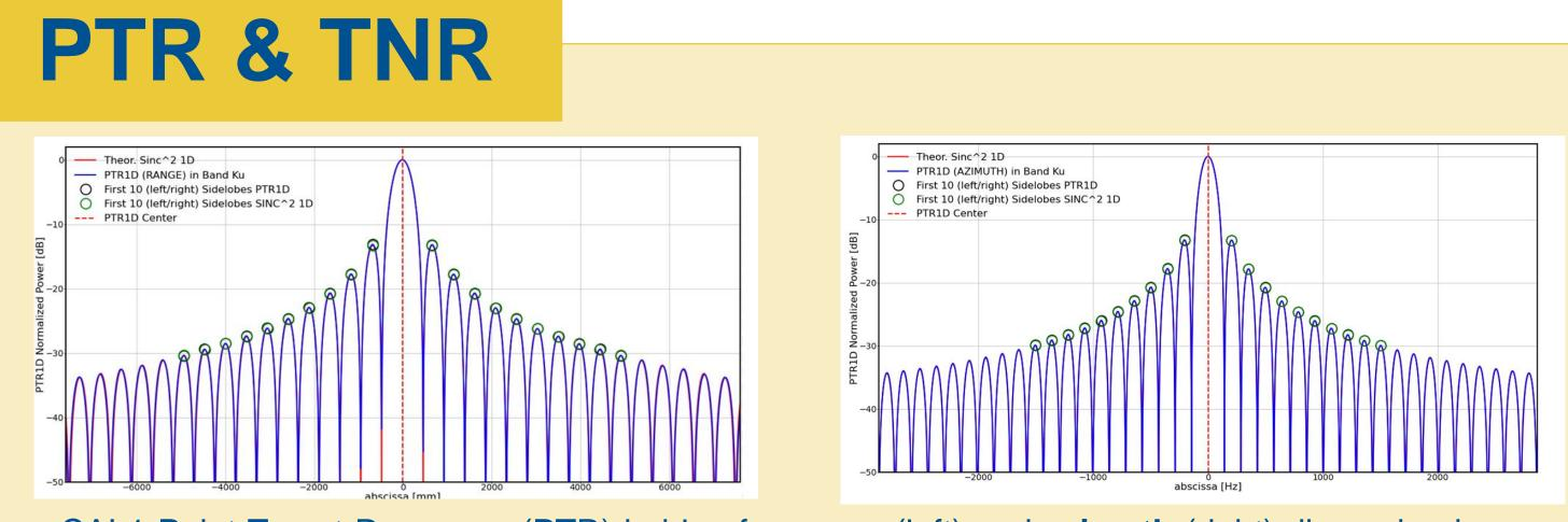
CAL1 Point Target Response (PTR) in blue for range (left) and azimuth (right) dimension in case of side-A Ku-Band. In red the ideal PTR (squared sinc) is displayed. Max side-lobe deviation is 0.22 dB in power and 7 mm in range
