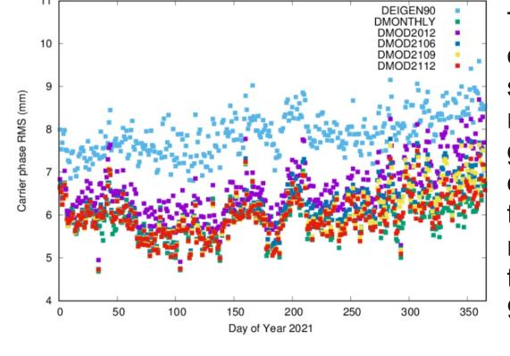
The carrier phase RMS of dynamic Sentinel-3B satellite orbits based on monthly GRACE-FO gravity fields (green) or different FSMs reveals the benefit of up-to-date models. All models were truncated at a max. d/o
