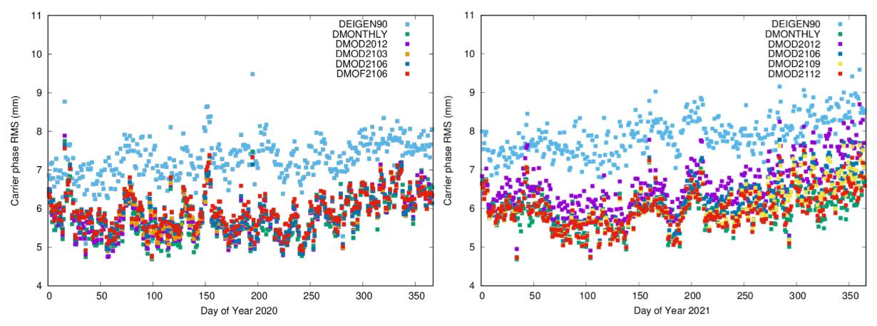
The carrier phase RMS of dynamic Sentinel-3B satellite orbits (orbit altitude 811 km) based on monthly GRACE-FO gravity fields (green) or different fitted signal models reveals the benefit of up-to-date models. All models were truncated at max. degree/order 90.
