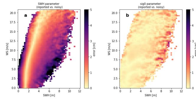
**Figure 2.** Jason-2, Ku-band SSB model error caused by (a) SWH uncertainty and (b) sig0 uncertainty. The SSB model errors for each independent variable error source at 2.5 m SWH and 7.5 m/s wind speed are (a) 0.945 cm and (b) 0.231 cm
