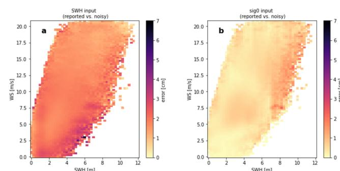
**Figure 4.** Jason-2, Ku-band SSB input error due to (a) SWH uncertainty and (b) sig0 uncertainty. The SSB input errors at 2.5 m SWH and 7.5 m/s wind speed are (a) 1.766 cm and (b) 0.67 cm
