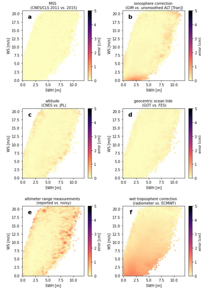
**Figure 1.** Jason-2 SSB model error corresponding to uncertainty in (a) MSS, (b) ionosphere correction, (c) altitude, (d) geocentric ocean tide, (e) altimeter Ku-band range measurements and (f) wet troposphere correction. The SSB model errors for each individual error source at 2.5 m SWH and 7.5 m/s wind speed are (a) 0.001 cm, (b) 0.073 cm, (c) 0.023 cm, (d) 0.014 cm, (e) 0.028 cm and (f) 0.458 cm.
