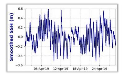
• Smoothed sea surface height from a 25 minute moving average filter to remove high frequency signals. From this, the tides, mean sea surface and inverse barometer has been removed to estimate sea level anomaly.
