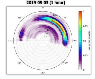
Directional spectra from the displacements in north and east, calculated over 5 minute segments and averaged over each hour.
