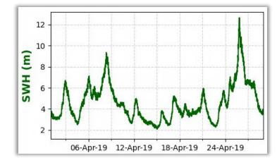
Significant wave height calculated as four times the standard deviation of clean 2 Hz SSH estimates over a rolling one hour window.
