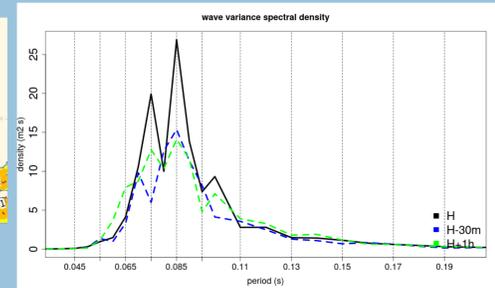
1D spectra observed by buoy at the hour H of rogue waves, just before (blue) and just after (green)
