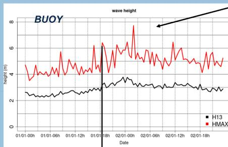
SWH of 3,1 m and Hmax of 6,4 m
