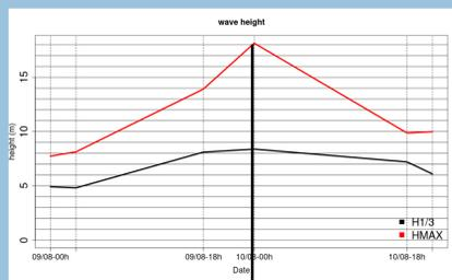
SWH of 8,4 m and Hmax of 18,1 m
