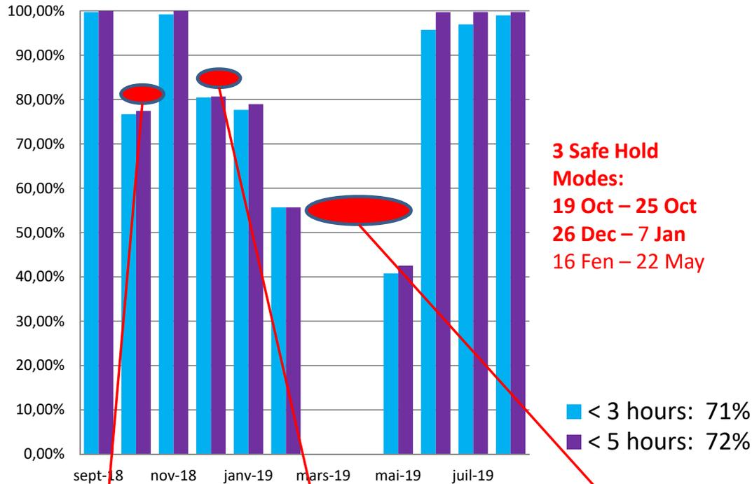
Anomaly with Gyro 2 triggered a satellite SHM (Safe Hold Mode). No OGDRs produced for subsequent passes.
