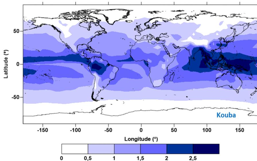
RMS (cm) of the WPD differences between 3-D and 2-D with reduction to the PL using different modelings, using profiles every 3-h in a grid 5°x5° over the year 2014 (not used in the UP modeling).
