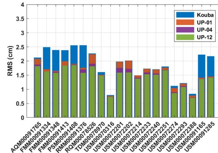
RMS (cm) of the WPD differences between RS and lowest level with different reductions, using soundings every 12-h over the year 2014.
