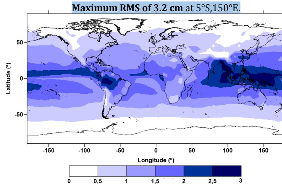
RMS (cm) of the WPD differences between 3-D and 2-D with Kouba reduction, using profiles every 3-h in a grid 5°x5° over the year 2014.
