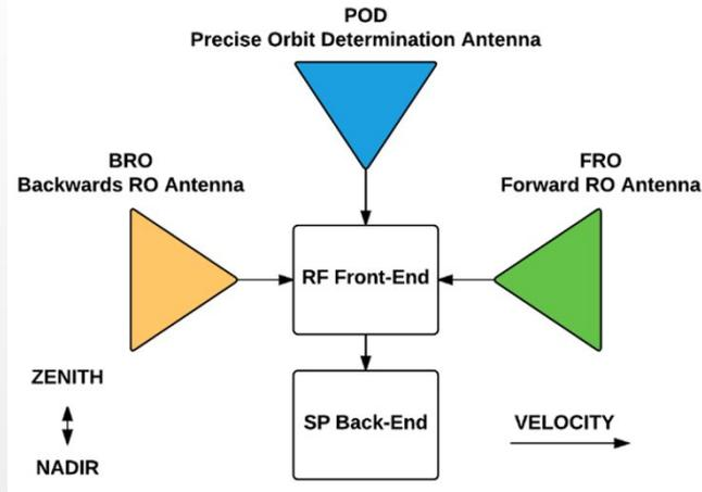
STRATOS is an advanced, software-defined, dual-frequency, low-power GNSS receiver for remote sensing and precise orbit determination (POD)
