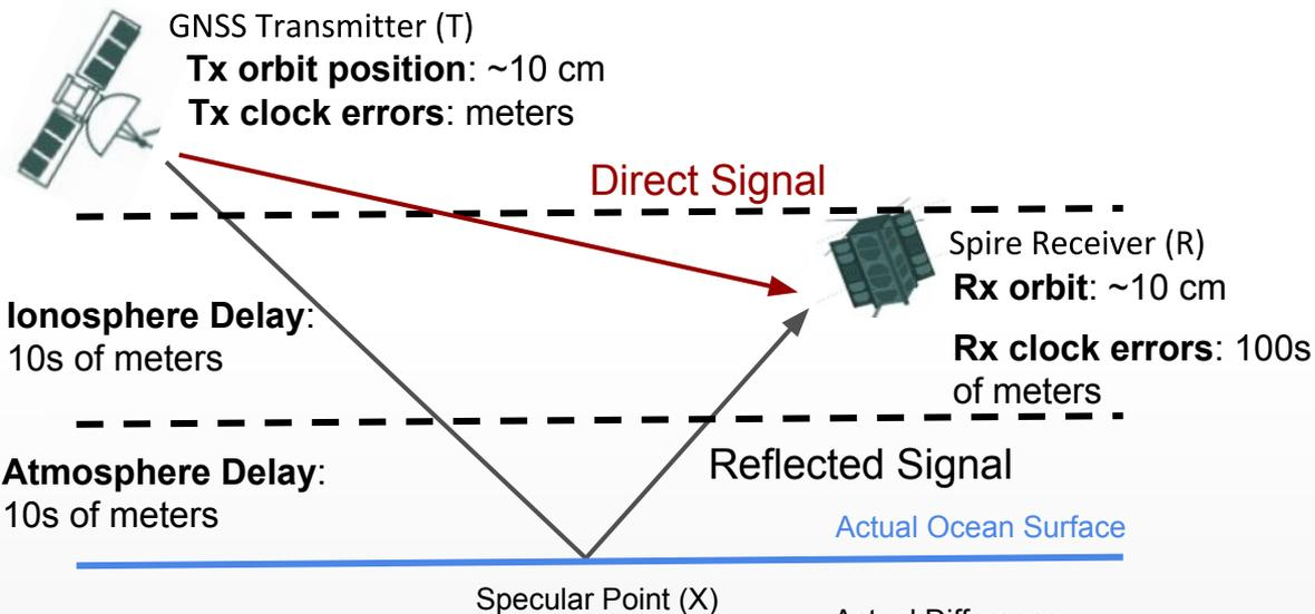
GPS pseudorange and phase measurements provide approximation of signal travel distance based on timing
