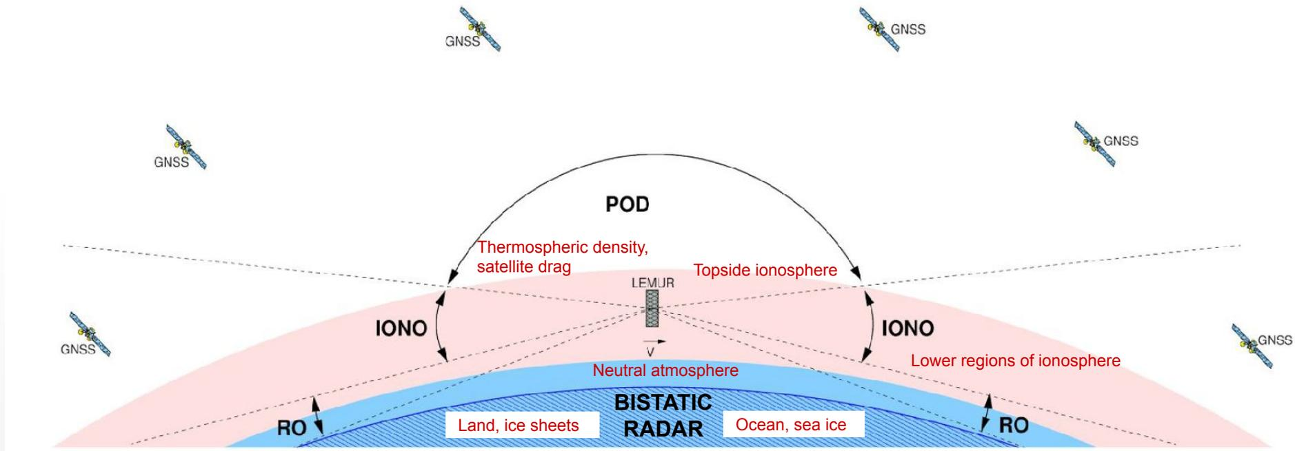
Spire leverages the ultra-stable, dual-frequency L-band signals broadcast by GNSS satellites to measure Earth properties that perturb these signals (e.g., refraction, **reflection**, etc.). These observations have various applications, such as NWP (radio occultation), space weather (TEC), **bistatic radar**, **altimetry**.
