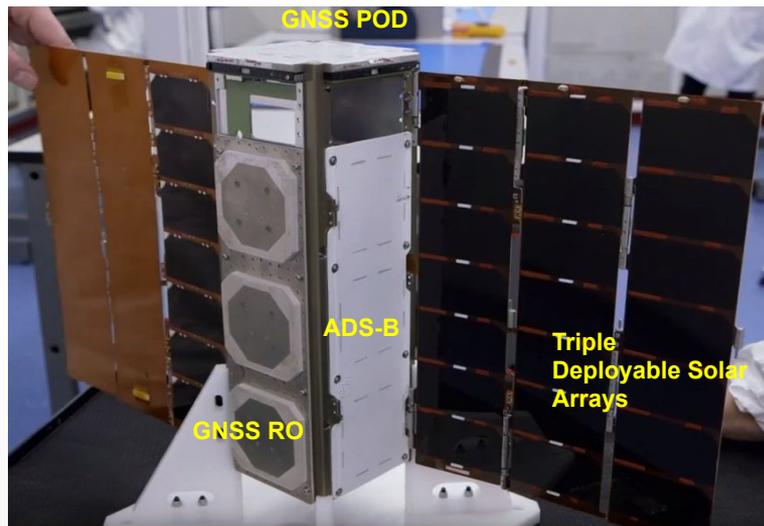
Spire designs and assembles nearly all of its satellite components in-house, ensuring expert-knowledge of the full satellite HW, SW, and processing stack
