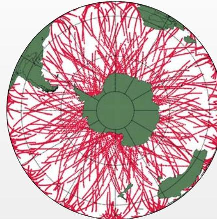
Coverage for 1 RO sat in sun synchronous orbit collecting GPS, GLONASS, Galileo, and QZSS reflections
