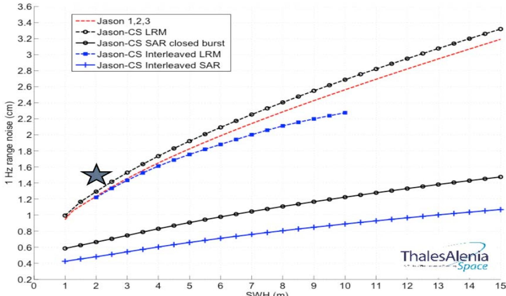
1-Hz altimeter range noise for closed and interleaved modes
