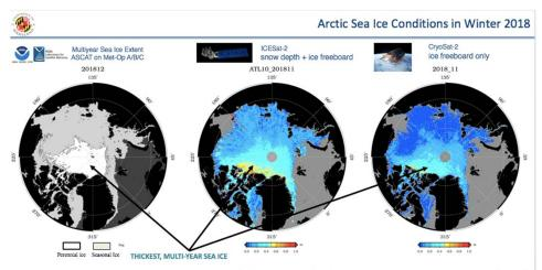
Independent, multi-sensor sea ice observations from ASCAT (left) and CryoSat-2 (right), show remarkable consistency with ICESat-2 (middle)
