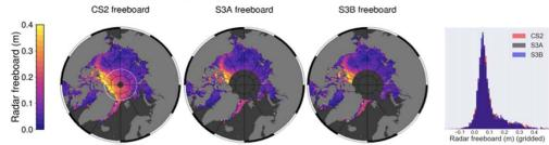
S3 Freeboard (Zero Padding, Hamming Applied) compared with CryoSat Freeboard: Lawrence et al, 2019
