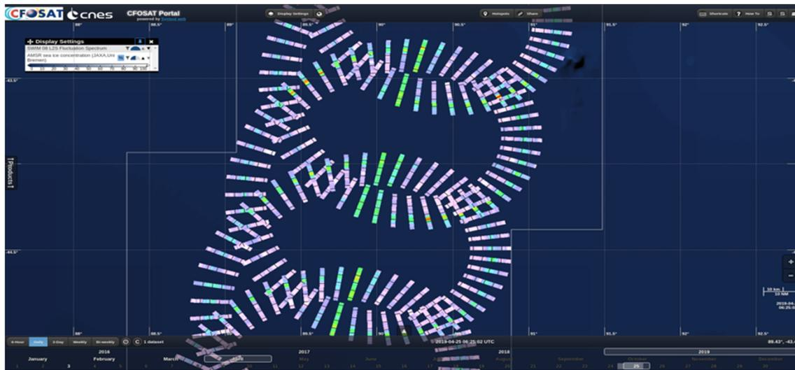
*example of radial density spectra (color codes) along the SWIM sampling (here 8° incidence beam)*
