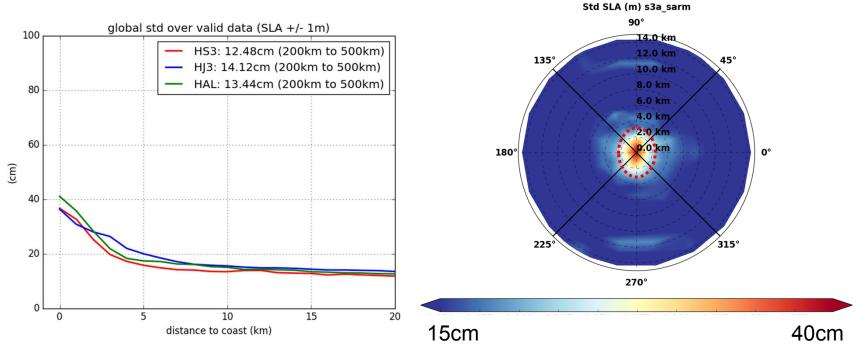
With the selection done on this study (remove only outliers >1m, chosen to keep significant number of points), SLA std computation at HR leads to global std of 12 to 14cm in average in open ocean (lower for S3a SAR mode than for lower resolution mode).
