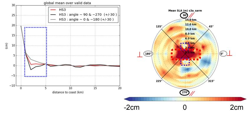
Impact on Sentinel-3 depends on attack angle to coast: Visible when satellite is moving // to the coast (footprint is of 15km length in cross track direction)
