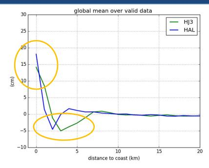
SLA mean drops then goes up when approaching coast mainly visible using LRM (AltiKa & Jason-3), due to land contamination in waveform.
