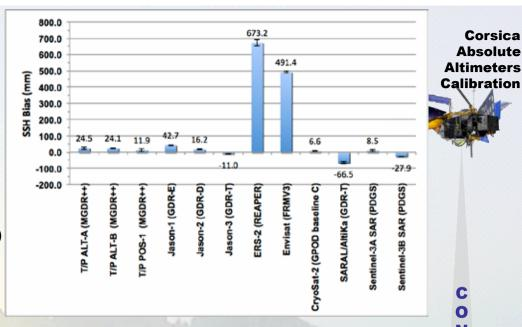
These new SSH biases are based on a complete update of Ajaccio and Senetosa geodetic datum and the most recent reprocessings of altimetry data sets.
