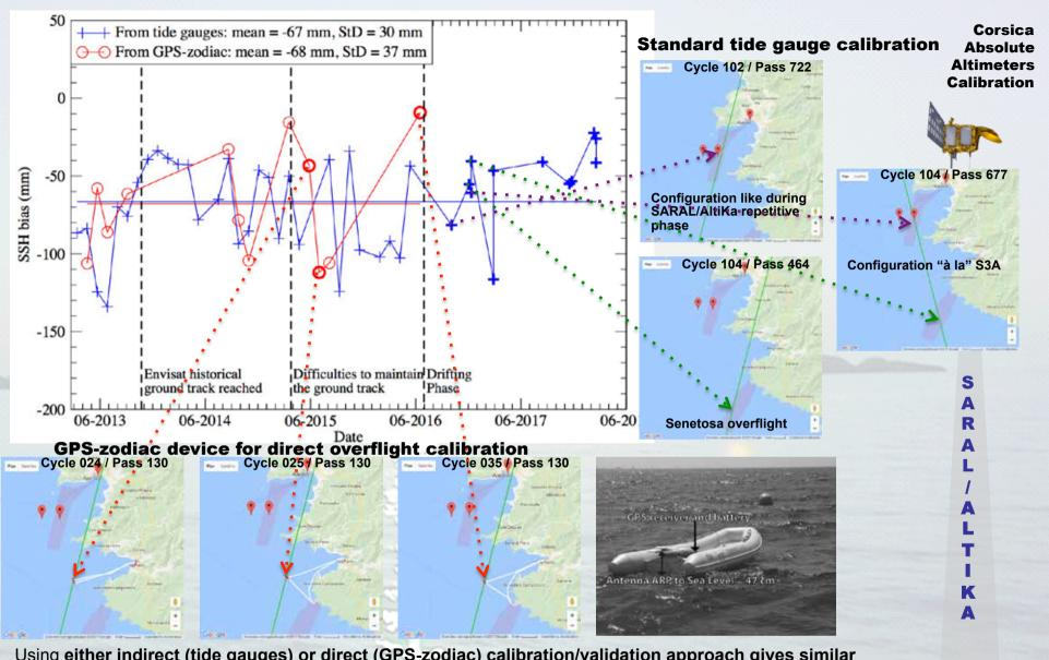
Using either indirect (tide gauges) or direct (GPS-zodiac) calibration/validation approach gives similar SSH bias, respectively -67 ± 5 mm and -68 ± 11 mm. Even during the Drifting Phase, we can continue to monitor the SSH bias using both approaches with a good agreement compared to the whole time series and a period close to the initial one: 36 days in average compared to the 35-day repeat period during the nominal phase, but not evenly distributed.
