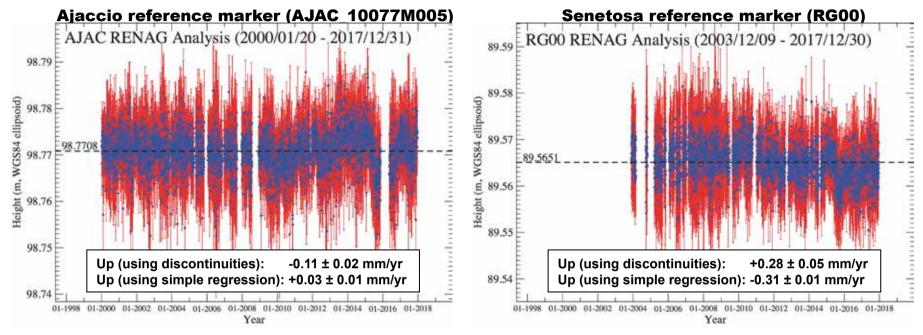
In the frame of the RENAG project (http://renag.resif.fr) a **complete reanalysis of the GPS coordinates has been performed** for the Ajaccio (AJAC) and Senetosa (RG00) reference markers **in the ITRF2014 reference frame**.
