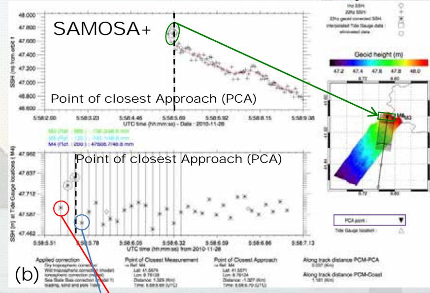
Some data very close to the coast (less than 500 m cross track, see red arrows) are clearly improved with SAMOSA+ (top frame: SSH; bottom frame: SSH corrected from geoid slope between altimetric point and tide gauge)
